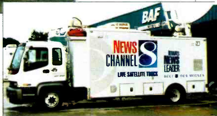
A large 'combo' truck BAF built for CBS affiliate kccv(tv) Des Moines, Iowa. The SNV-210T dual-path SNG truck has a 42-foot microwave mast.
